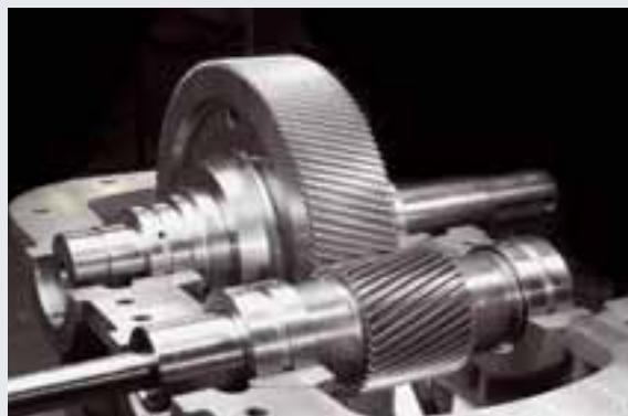
View inside a gearbox
