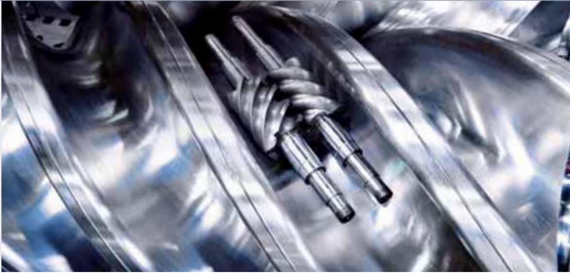
Smallest and largest screw compressor rotors made by MAN Diesel & Turbo
