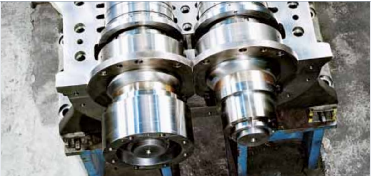
Combined journal and thrust bearings of male and female rotor
