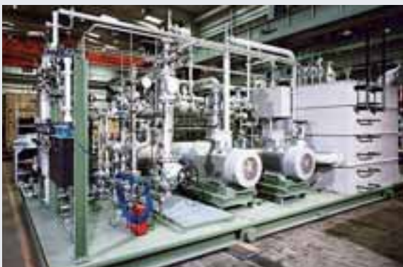
Separate oil supply console designed according to API 614
