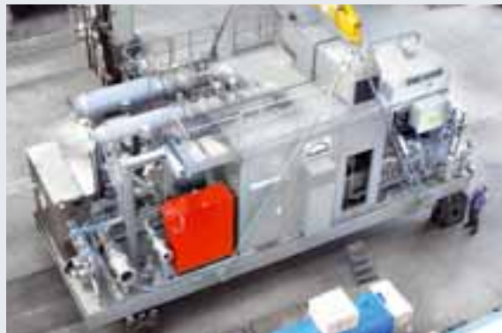
View of a process-gas screw compressor module for an offshore application
