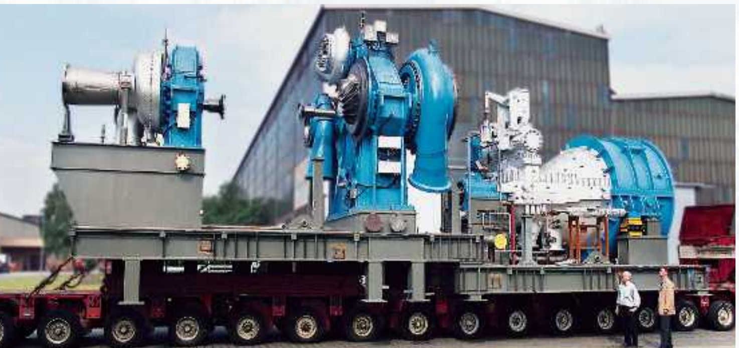
12 Machine set of a PTA plant with steam turbine and expander drive
