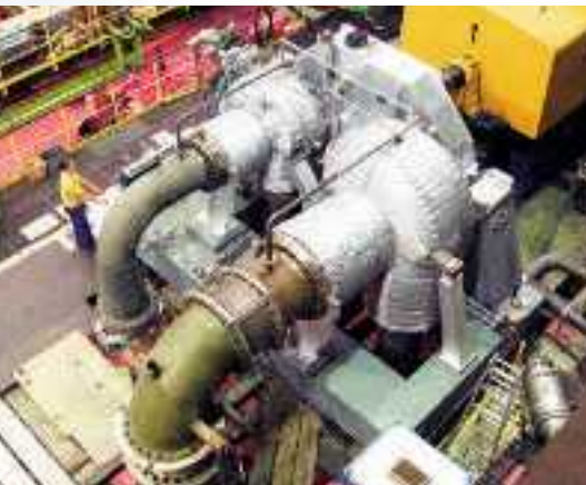
14 High-temperature expander in multi-shaft (integrally-gear) technology, 2 radial-inflow stages
