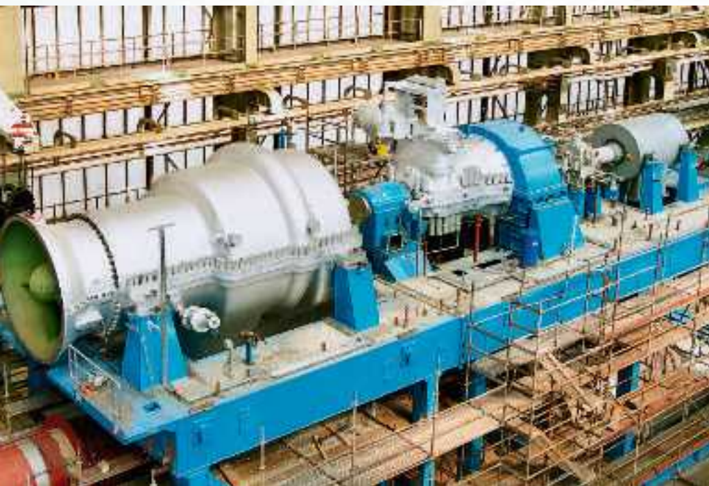
25 Machinery train for an air separation plant in the GTL process, works test assembly
